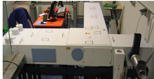
**MIS-DL** –Michelson interferometer stabilized diode laser. The instrument has been upgraded in 2011 and installed during 2012/2013. It consists out of a tunable laser source (TDL) coupled to a Michelson interferometer which is stabilized by a HeNe laser. Spectra over the DL tuning rates can be obtained at high spectral resolution.
