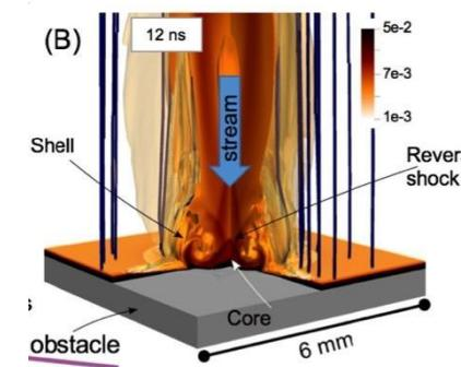
3D simulation of the ELFIE laser experiment with GORGON (Revet & al. Science Adv. 2017)
