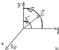
$$n^{2} = 1 - \frac{\omega p^{2}}{\omega(\omega - \omega_{B})} \quad \text{et} \quad n^{2} = 1 - \frac{\omega p^{2}}{\omega(\omega + \omega_{B})}$$
